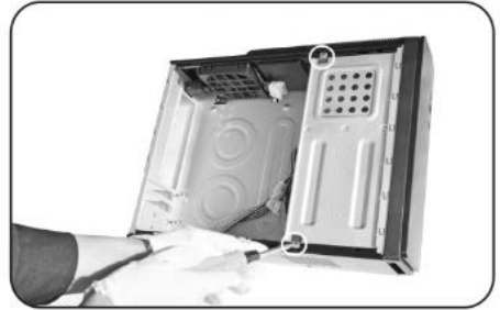
2 – Lies the case on the tabletop Twists off two screws on the 5"25 bay.
