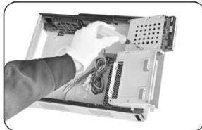
6 – Installs the hard disk.
