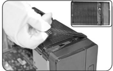
4 – Install and uninstall power supply may take out of the obstruct piece on the top panel.
