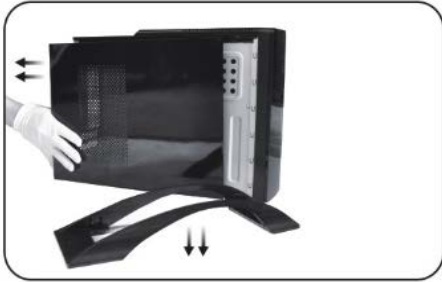
1 – Takes down the foot Twists off the screw on the rearpanel to take down the side panel
