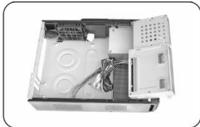
5 – Puts slanting 5"25 bay revolution axis position on the rack.
