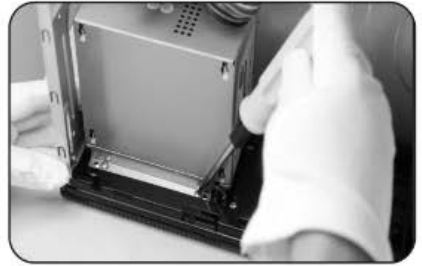
2 – Remove 2pcs screw, take down power supply.
